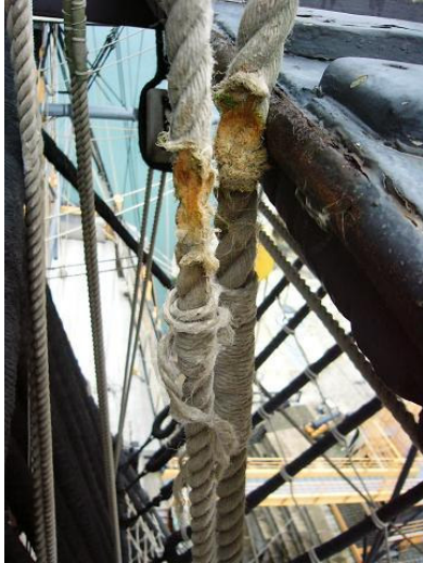
Even in non-seagoing rigging chafing can be disastrous.
